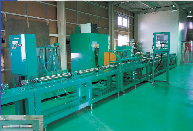
▼ CNC MF. INDUCTION M/C (JAPAN)
