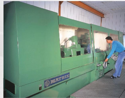
▼ EXTERNAL THREAD GRINDER (U.K.)
