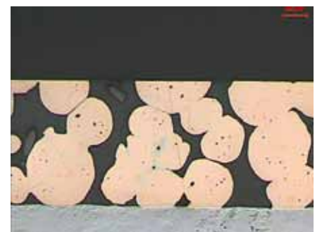
Fig. 8: Condition of sliding surface during service life
