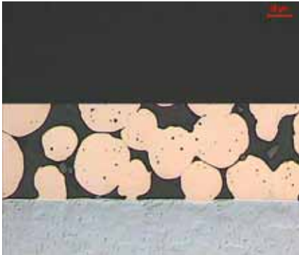
Fig. 9: Condition of sliding surface at end of service life
