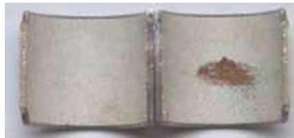
Fig. 34: Local damage caused by cavitation
