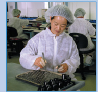
Class 1000 Clean Room
