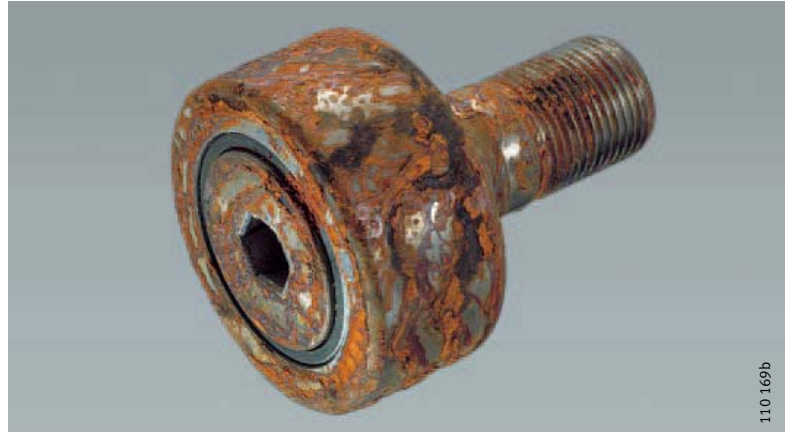
Figure 1 NUKR52 without coating after salt spray test
