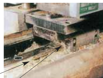
Wood chips Linear guide equipped with high-performance seal
