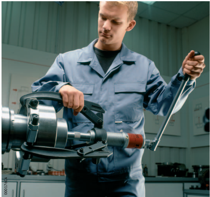
Figure 1 Dismounting of a bearing using a hydraulic extractor
