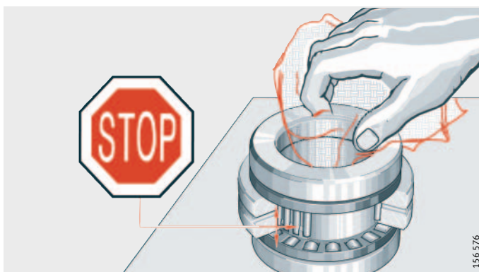
Figure 3 Cleaning of bearings
