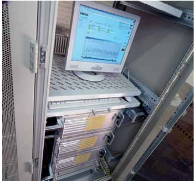
Figure 10 Condition-based rolling bearing monitoring using FAG VibroCheck
