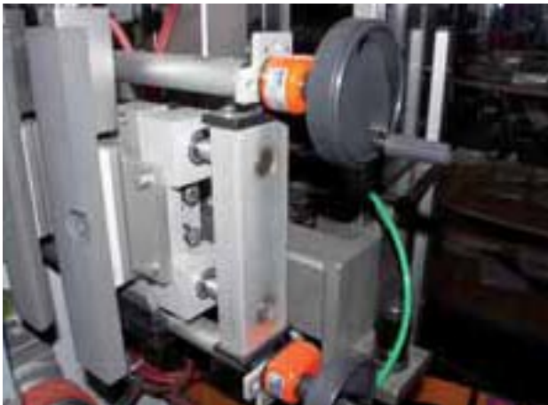
Format adjustment using DryLin® Easy Tube
