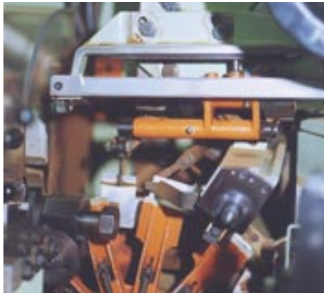
Picture 7.1: By converting to iglide® L280, the life of the bearing on this tea bag packaging machine was increased five times
