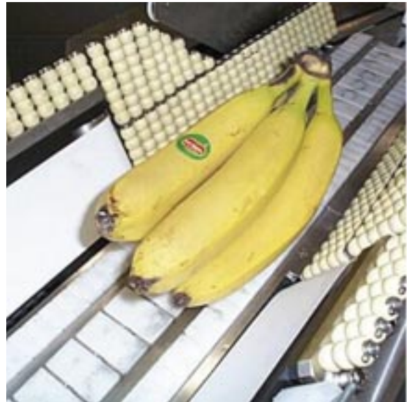
igubal® spherical balls in the food industry
