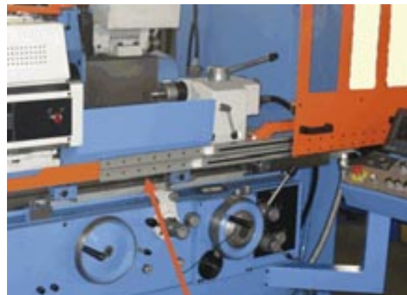
DryLin® NT-LM in guard door adjustment in machine tool
