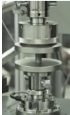
Testing of the compressive strength of iglide® plain bearings
