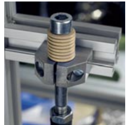
Polysorb Disc Springs in a fatigue test
