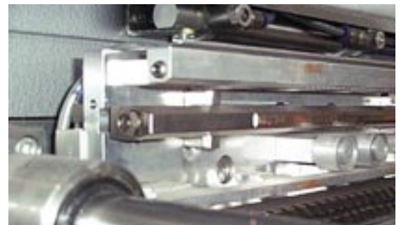
DryLin® high-temperature bearings made of iglide® T500 are used to support the sealing bar in this packaging machine. The TUM liners run without lubrication at temperatures of around 266°F, allowing a class leading output of 90 cycles/min.
