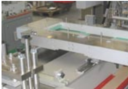
Feeding systems for a blister machine
