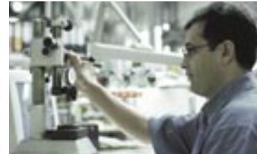
Measurement of the inner diameter of a pressfit plain bearing
