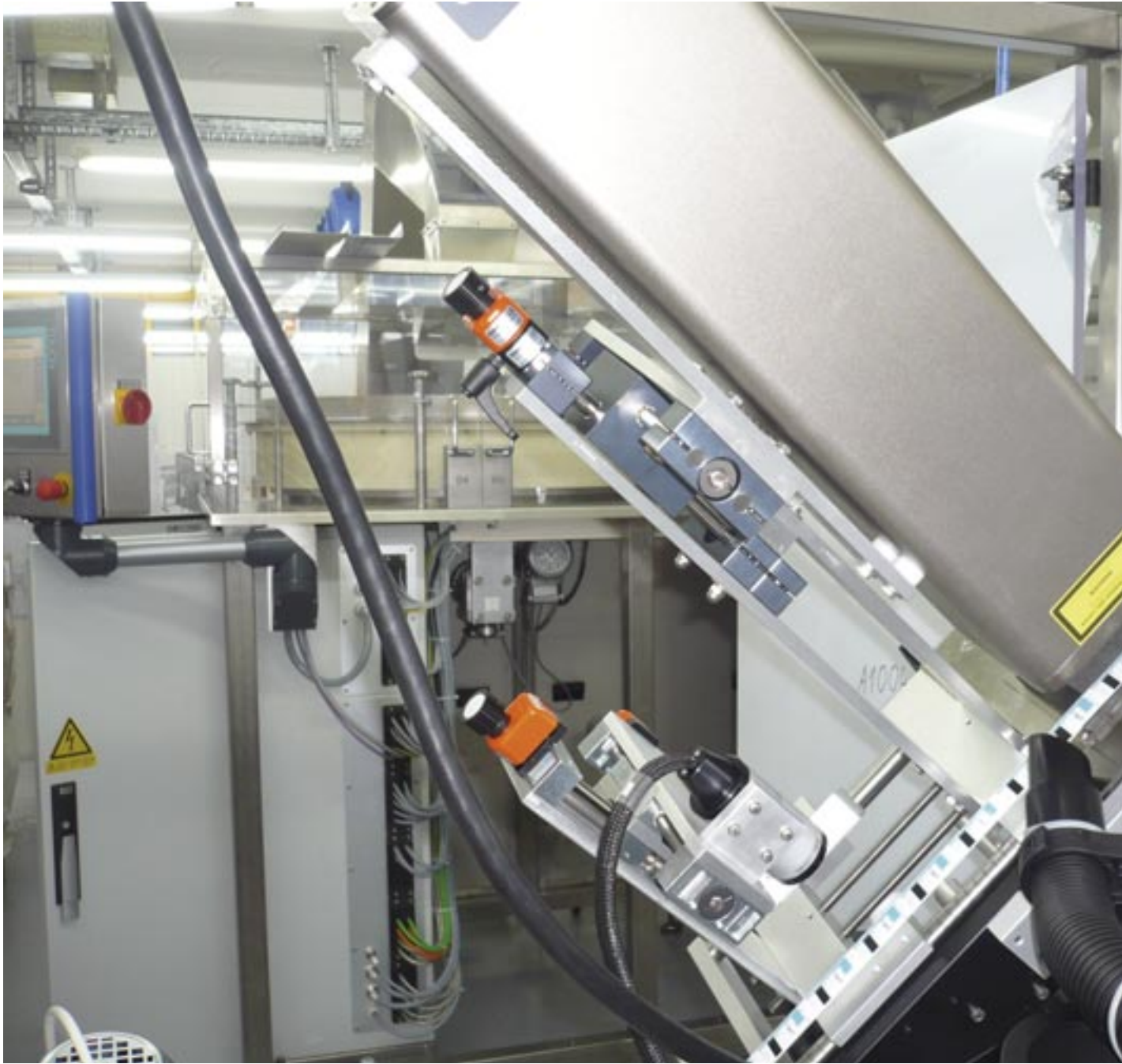
HTs and SLWE-XY in a camera/laser adjustment inspection application
