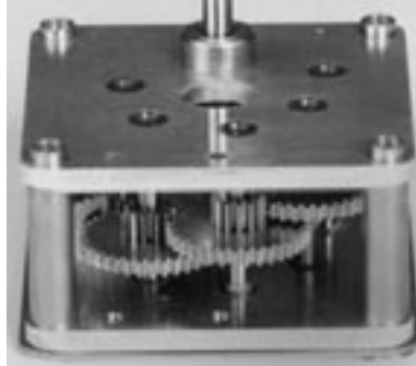
Picture 2.2: Precision mechanical gears need plain bearings with especially universal properties
