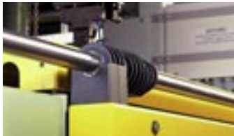
DryLin® R linear bearings in a safety door
