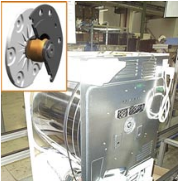
Drum bearing in a tumble dryer
