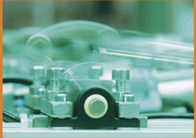
Above is a test to determine the maximum running speed of an igubal® pillow block bearing.
