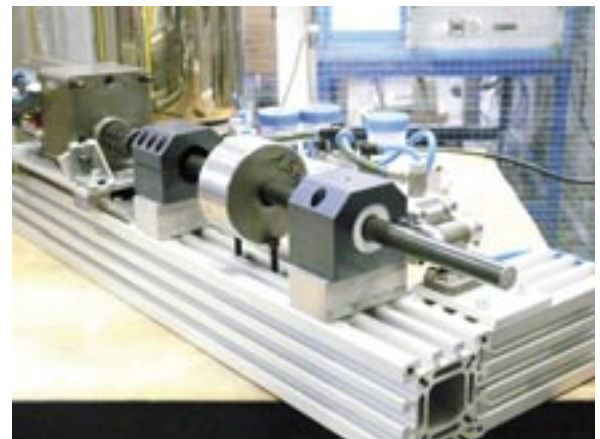
Test benches for xiros® plastic ball bearings at igus® laboratory
