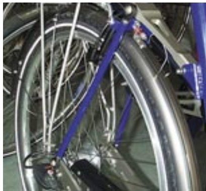
igubal® rod end bearings in the spring loaded rear axle of a bicycle
