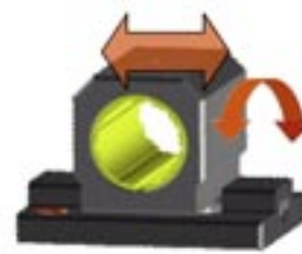
The self-aligning DryLin® R bearings of the 06 LL design series can compensate parallelism errors up to ± .12" (3mm).
