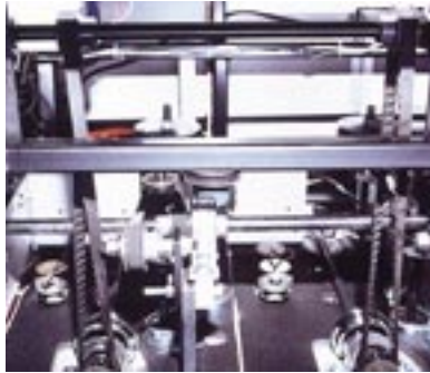
Picture 2.1: Paper dust in this mail sorting device always led to an early malfunction of the previous bearings used. Problem solved.
