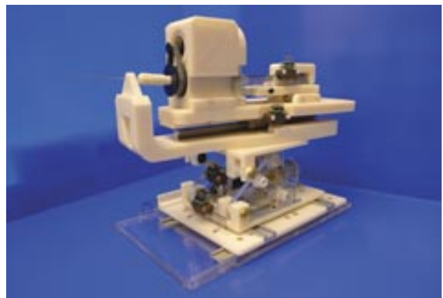
A PhD student from the Worcester Polytechnic Institute used DryLin® linear bearings and iglide® plastic bearings to facilitate motion on this MRI-guided robot, which will revolutionize the way prostate cancer is detected and treated.
