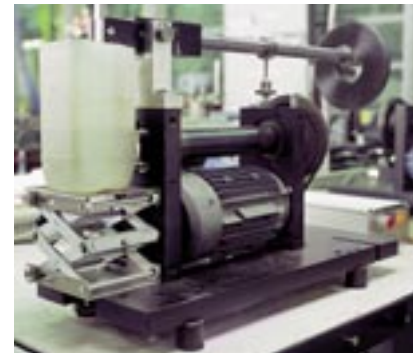
Rotational testing stand for underwater and/or chemicals
