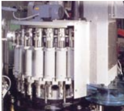
Picture 10.1: Filling applications: linear, oscillating, and rotating movements can be achieved using iglide® H370 bearings
