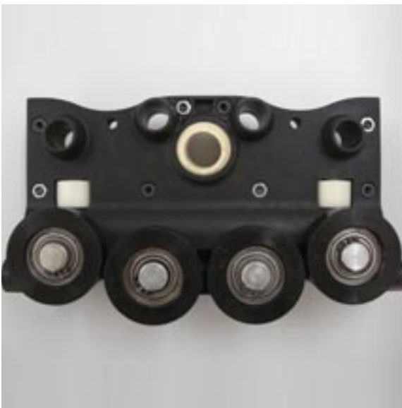
Carriage in a crane system
