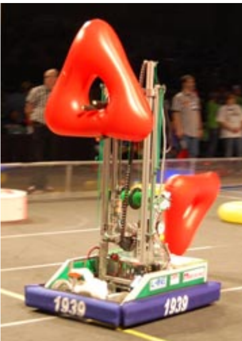
For this FIRST® Robotics team, DryLin® linear guides and iglide® plastic bearings were a lightweight alternative to metal or bronze bearings and facilitated movement for the robot's forklift.
