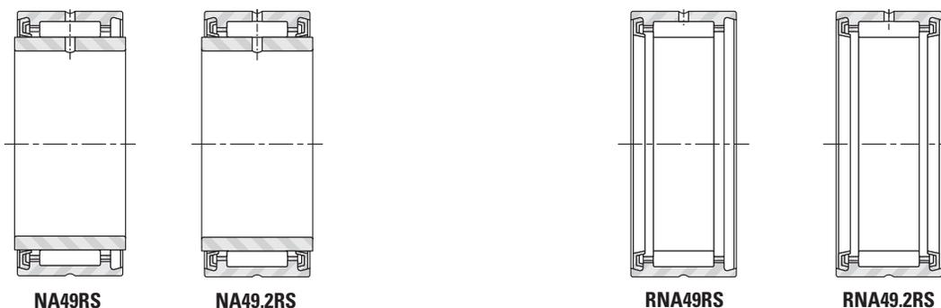
Fig. B-38. Sealed needle roller bearings with inner rings
