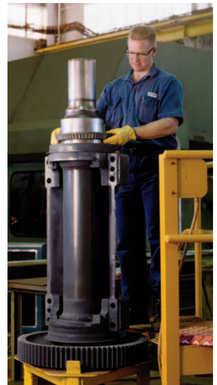
Mounting of a suspension tube roller bearing
