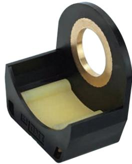
IKO C-Lube Unit for Cam Followers is a lubricating part to be mounted in Cam Followers. Periodic lubrication is not required because this product supplies the lubricating oil that is indispensable for the external diameter surface of the outer ring and track surface of Cam Followers.
