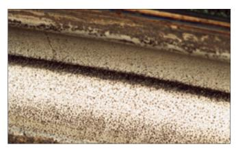
Photo 7-9-1Part:Outer ring of a slewing bearingSymptom:Pitting occurs on the raceway surfaceCause:Rust at bottoms of indentations
