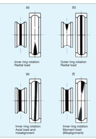
Fig. 6.1 Typical running traces of deep groove ball bearings
