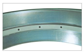
Photo 7-8-2Part:Outer ring of a double-row tapered roller bearingSymptom:Indentations on raceway surfaceCause:Debris caught in the surface
