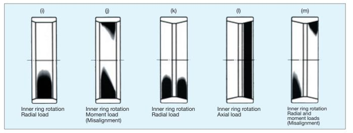
Fig. 6.2 Typical running traces on roller bearings
