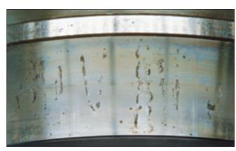
Photo 7-16-3Part:Inner ring of a spherical roller bearingSymptom:Rust on raceway surface at roller pitchCause:Entry of water into lubricant
