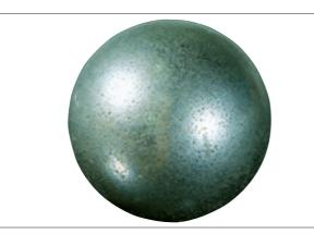
Photo 7-9-2Part:Ball of Photo 7-9-1Symptom:Pitting occurs on the rolling element surface
