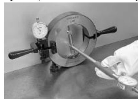
Fig. 1.11 Adjust the Inscribed Diameter of the GN Gauge
