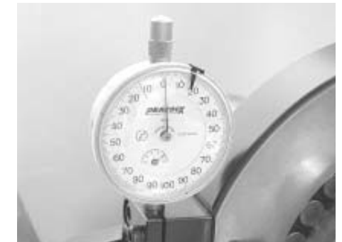
Fig. 1.15 Measurement of Spacer Width
