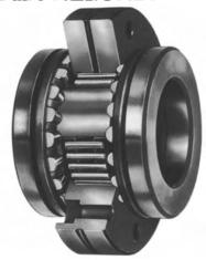
Types AXNA, AXNB and ARNB combined bearings and their derivatives consist of a needle bearing with or without a cage, in an outer race, with a high radial thickness, each face of which acts as a raceway for a needle or roller thrust bearing. The inner ring, secured laterally between the thrust plates, acts as the inner radial raceway.
