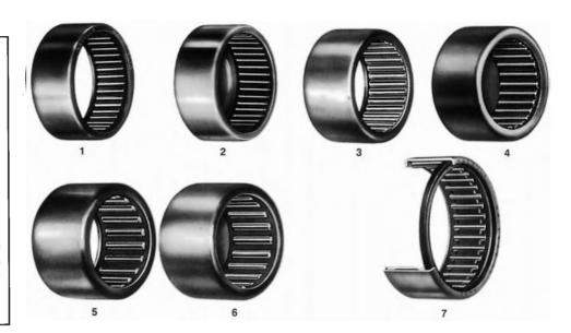
Needle bushes consist of a thin, heat treated outer ring formed from accurately controlled sheet steel encasing a set of needles. Bushes may have a full complement of needles retained in the outer ring by their ends or by grease; others have the needles retained in a cage which is prevented from moving laterally in the outer ring.
