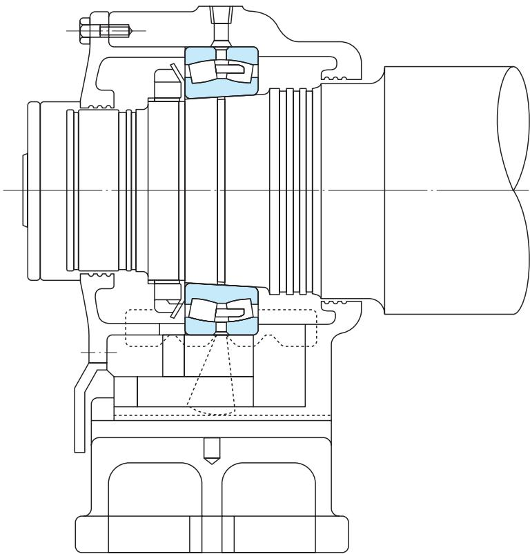
Figure 17 Dryer Roll, Paper Making Machine (Free End)
