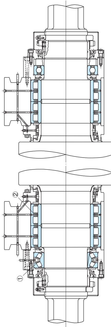
**Figure 7 Horizontal Roll Chock Assembly, Large-Size Universal Rolling Mill**
