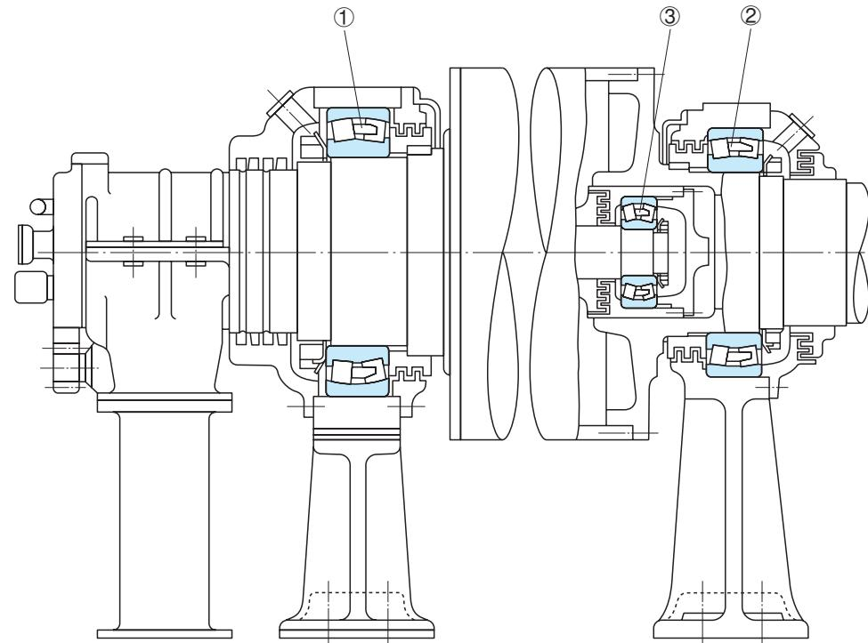
Figure 16 Suction Roll, Paper Making Machine
