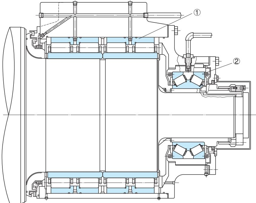
Figure 5 Back-Up Roll Chock Assembly, Cold Strip Rolling Mill
