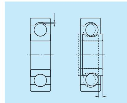
**Fig. 3.1 Bearing Internal Clearance**
