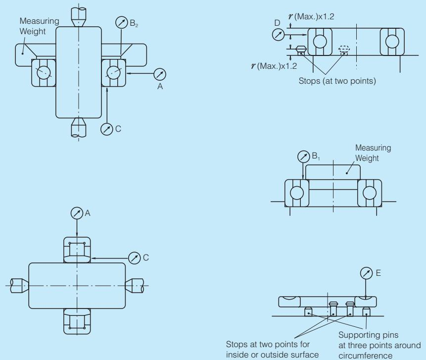
Fig. 2.1 Measuring Methods for Running Accuracy (summarized)
