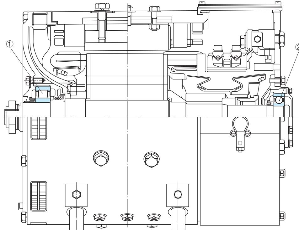
Figure 14 Traction Motor, Bullet Train (SHINKANSEN)
