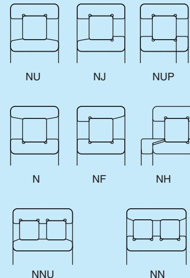
Types NU, N, NNU, and NN are suitable as free-end bearings. Types NJ and NF can sustain limited axial loads in one direction. Types NH and NUP can be used as fixed-end bearings. Loose rib for NUP inner ring should be mounted so that its marked side faces outward.
