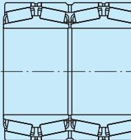
This type of bearing has two double-cone assemblies, two cups, one double cup, and three spacers. The bearings have their internal clearance adjusted for each set, so it is necessary to assemble them correctly in accordance with their serial numbers and matching symbols.
