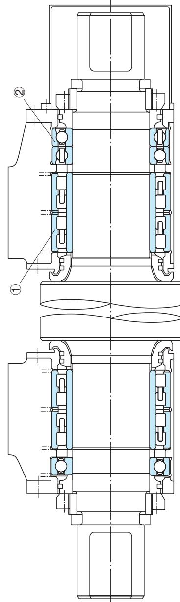
**Figure 8 Finishing Roll Chock Assembly, Wire Rolling Mill**
