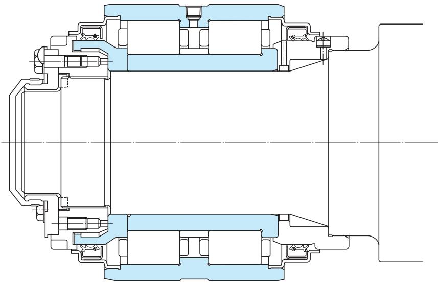
Figure 13 Axlebox Bearing, New Commuter Train
