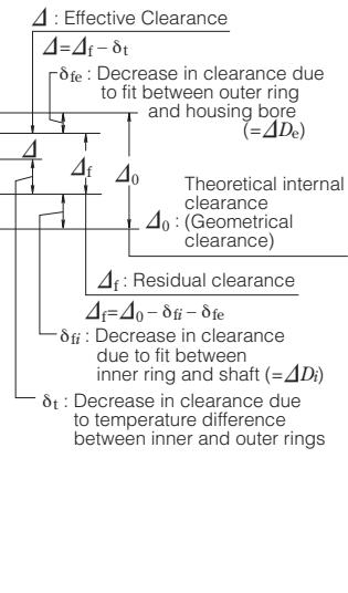
**Fig. 3.2 Change in Radial Internal Clearance of Bearings**
