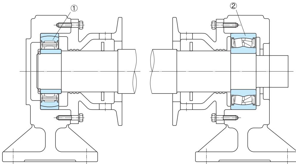
Figure 3 Table Roller, Hot Strip Rolling Mill
