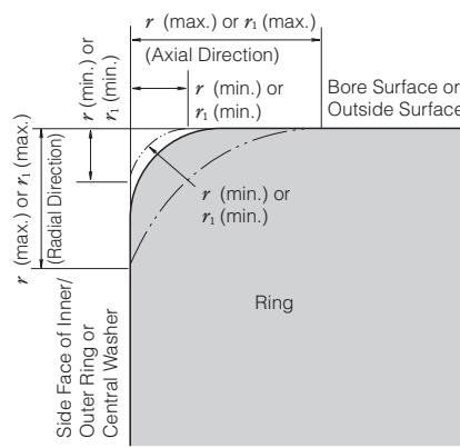
$r$  : Chamfer Dimension of Inner/Outer Ring
