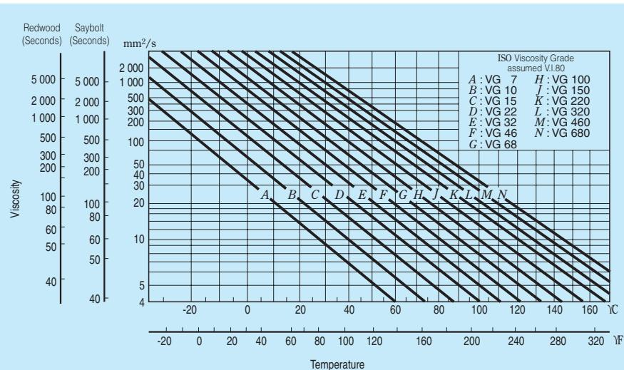
**Fig. 4.10 Temperature-Viscosity Chart**
