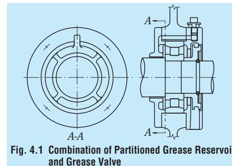
**Fig. 4.1 Combination of Partitioned Grease Reservoir and Grease Valve**
