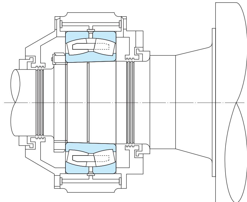
Figure 18 Press Roll, Paper Making Machine (Fixed End)
