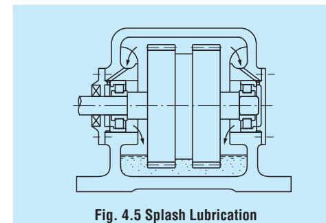
Fig. 4.5 Splash Lubrication
