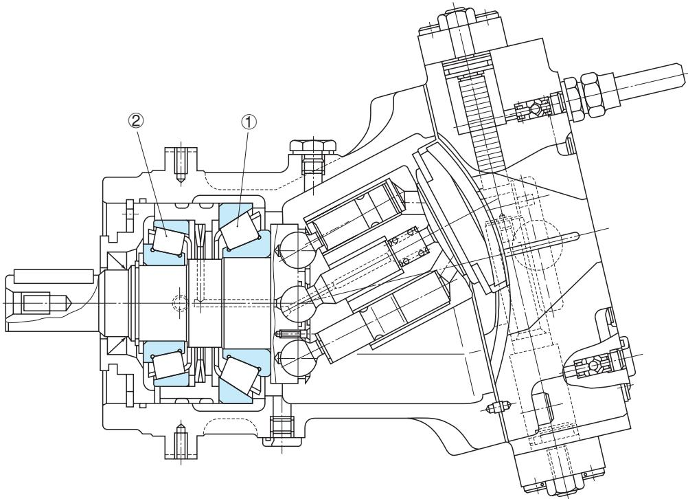
Figure 11 Bent Axis Type Axial Piston Pump
