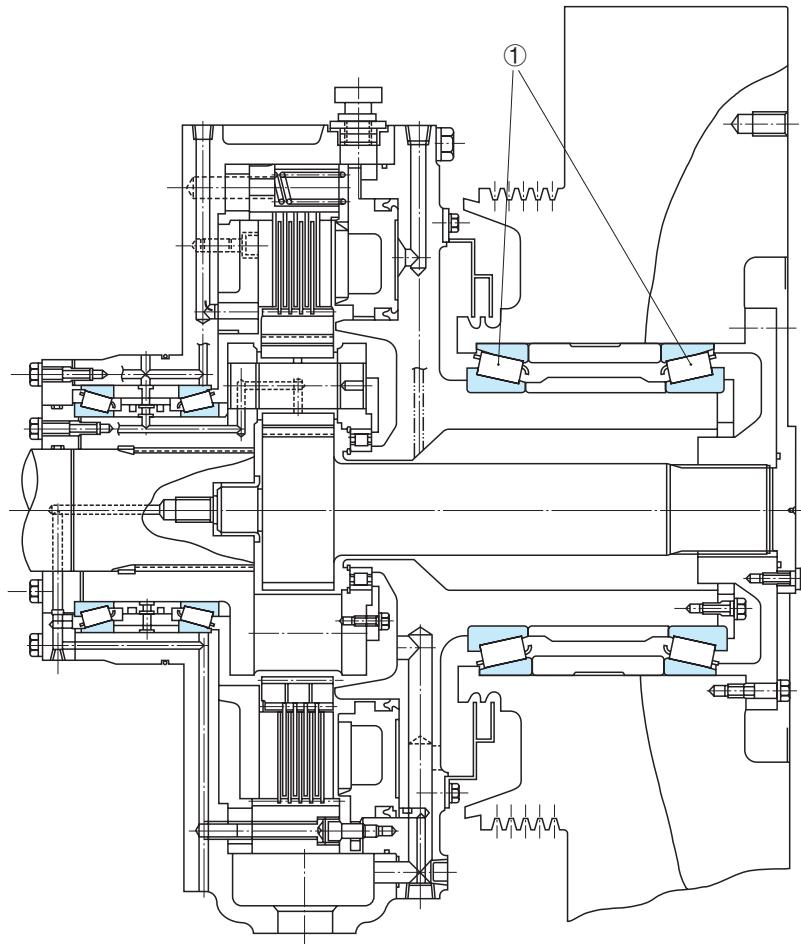
Figure 15 Flywheel and Clutch Assembly, Large-Size Press
