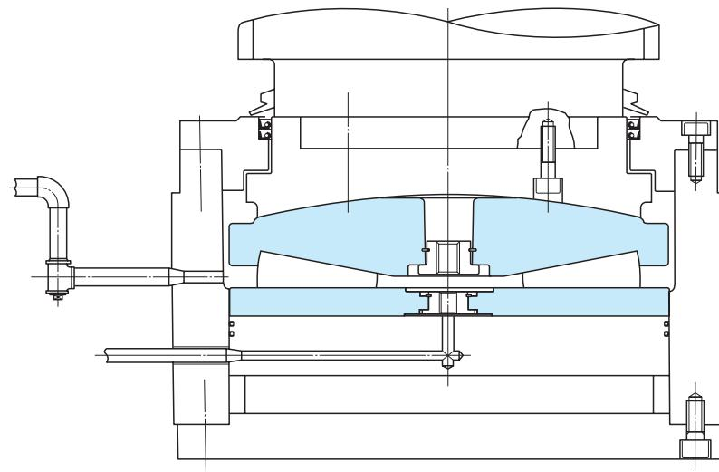
Figure 2 Adjusting Screw Thrust Block, Hot Strip Rolling Mill
