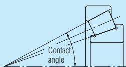
Tapered roller bearings are designed so the apices of the cones formed by the raceways of the cone and cup and the conical rollers all coincide at one point on the axis of the bearing. When a radial load is imposed, an axial force component occurs; therefore, it is necessary to use two bearings in opposition or some other multiple arrangement.
