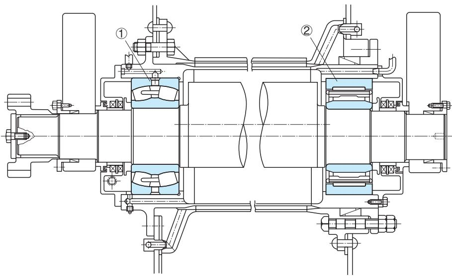
Figure 1 Eccentric shaft, Vibrating Screen
