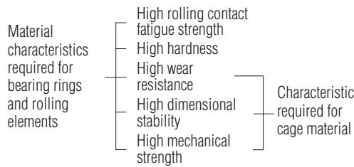
Other necessary characteristics, such as easy production, shock and heat resistance, and corrosion resistance, are required depending on individual applications.
