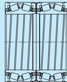
Basic Design of Four Seal Type
