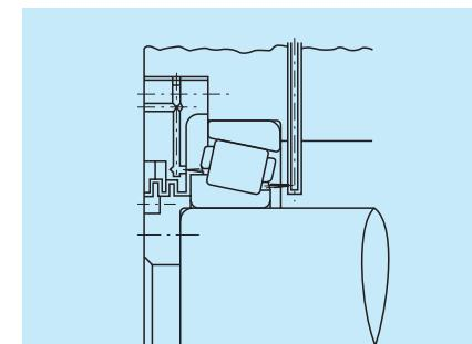
Fig. 4.7 Jet Lubrication
