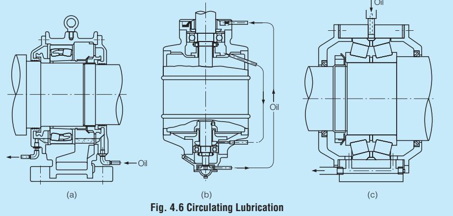
Fig. 4.6 Circulating Lubrication
