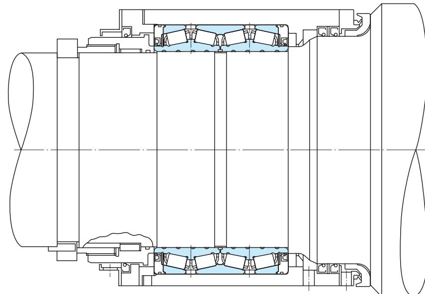
Figure 6 Work Roll Chock Assembly, Cold Strip Rolling Mill
