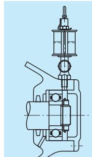
Fig. 4.4 Drip Feed Lubrication
