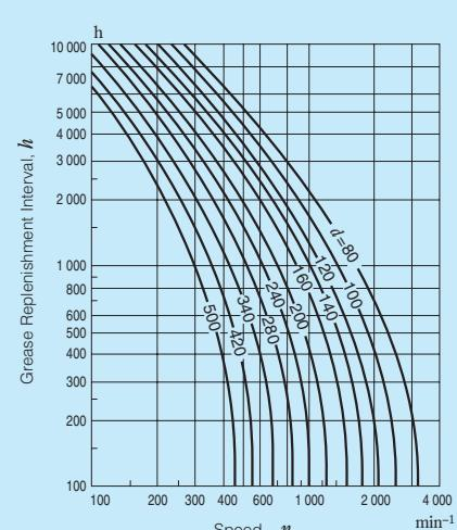
(2) Tapered Roller Bearings, Spherical Roller Bearings
