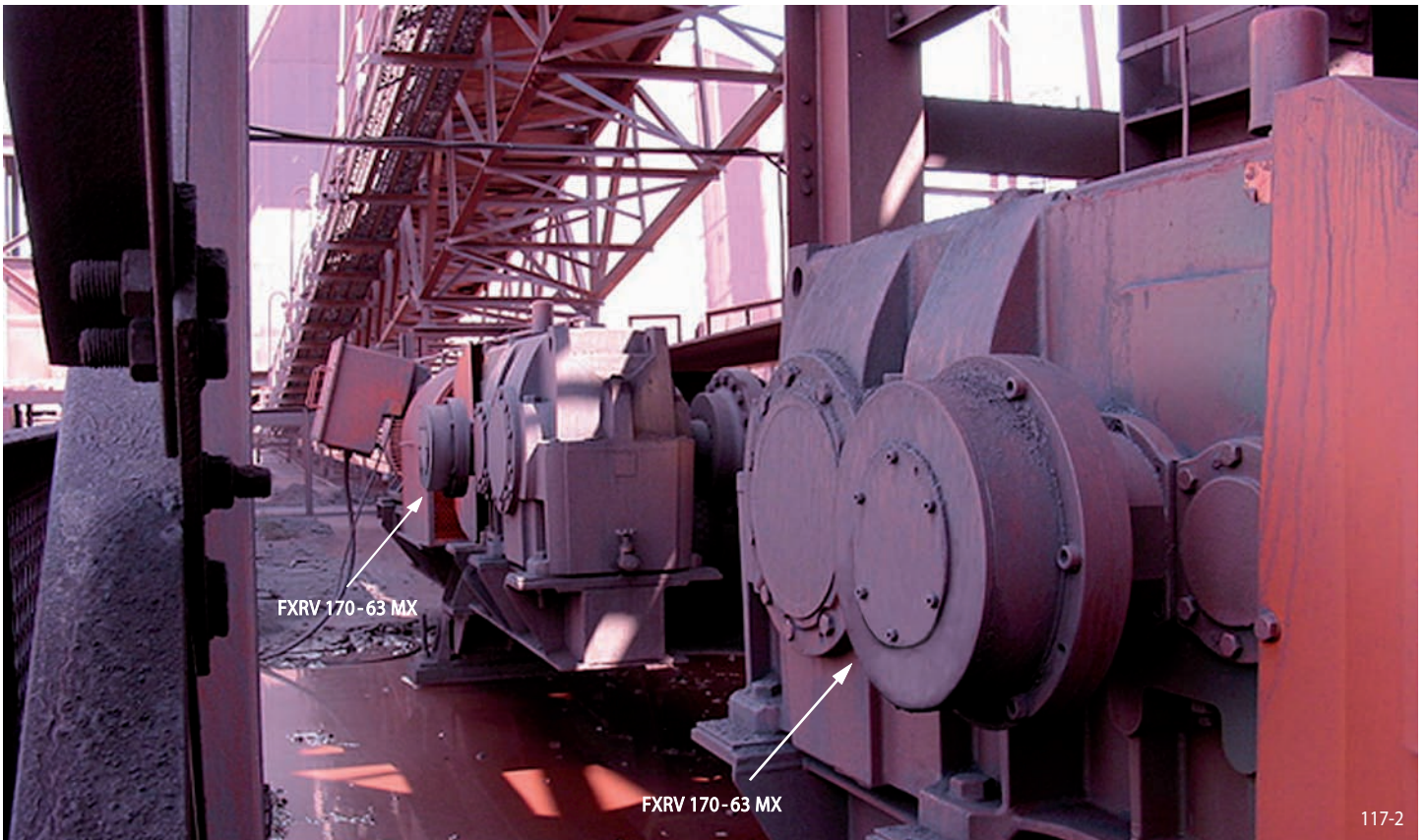
Iron ore conveyor plant in South Africa driven by three gear reducers with RINGSPANN backstops FXRV 170 MX.
