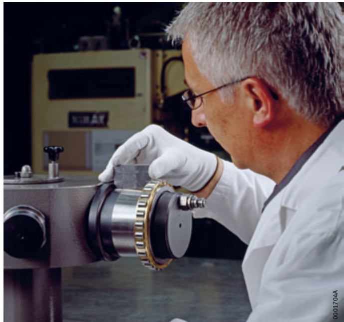
Figure 5 Measuring the distance to the shaft shoulder
