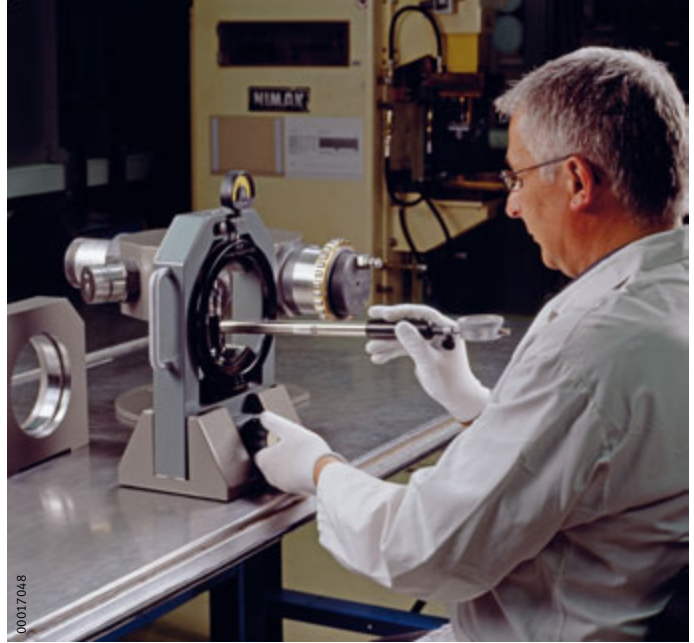
Figure 3 Transferring the raceway diameter to the enveloping circle gauge
