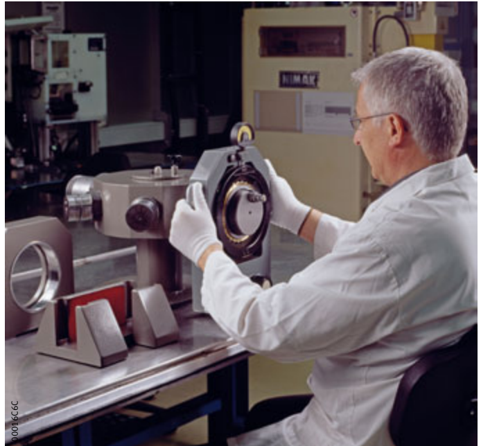
Figure 4 Positioning the enveloping circle gauge
