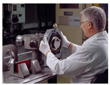
Figure 3 Positioning the enveloping circle gauge
