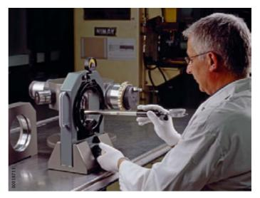
Figure 2 Transferring the raceway diameter to the enveloping circle gauge
