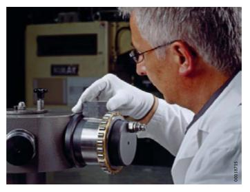
Figure 4 Measuring the distance to the shaft shoulder
