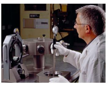
Figure 1 Raceway diameter of the outer ring
