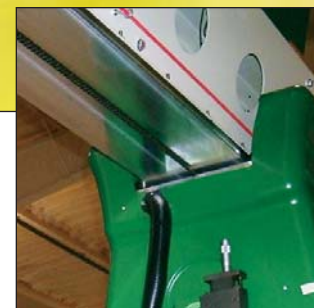
Inverted IVT linear guide assembly.
