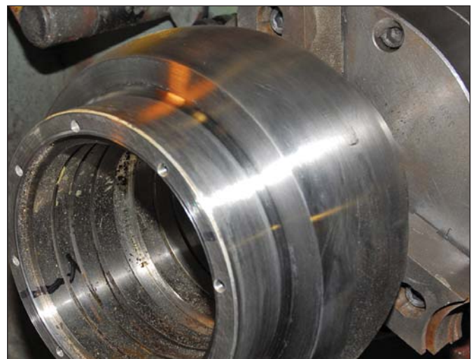
PBC Linear Doctor Bearing after 16 years of performance.
