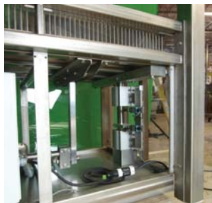
The bed-of-nails lift table requires linear guidance capable of handling loads up to 1000 lbs.
