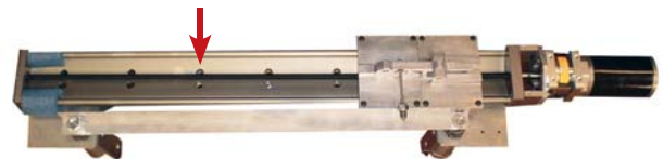
Uni-Guide assembled into kicking mechanism
