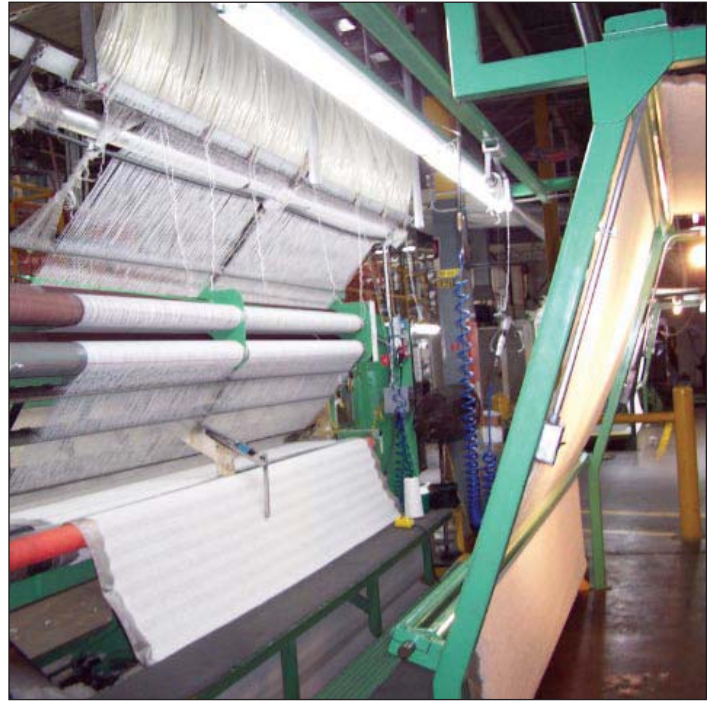
Carpet tufting machine with Simplicity® assembly installed at the feet.
