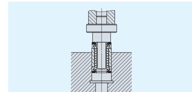
Fig.5 Press-fitting of the external cylinder
