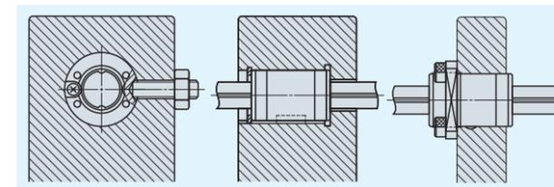
Fig.3 Mounting example of external cylinder
