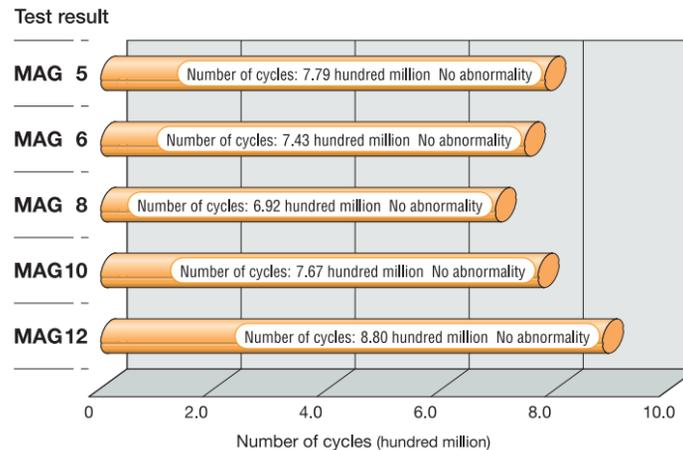
At vertical shaft and super high tact operation, the product can endure at the total number of reciprocating motions of 2 hundred million without any trouble only with the oil prepacked in the C-Lube. Maintenance free operation equivalent to the period of 10 years has been achieved in the test conditions supposing the operating conditions for general chip mounters.
