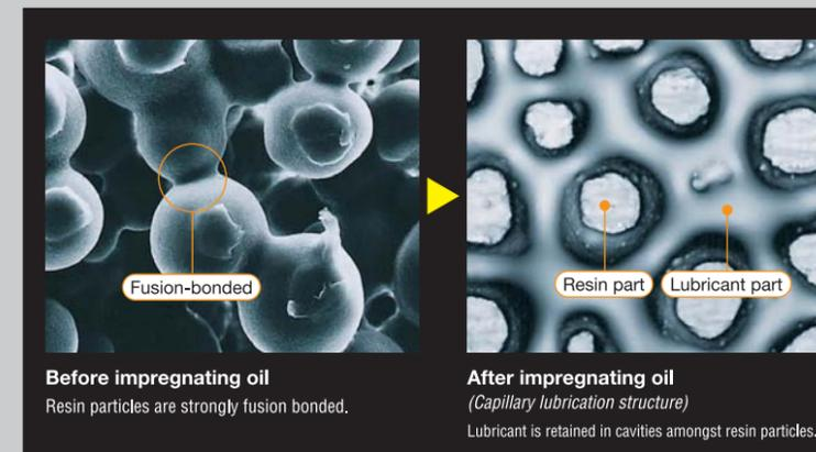
Capillary system IKO has developed is a new type lubrication. It is a porous resin Lube-body or plate with steel backing formed by sintering fine resin powder and impregnating a large amount of lubrication oil in its open pores. Capillary system always supplies proper amount of lubrication oil to the cylindrical rollers and lubrication condition of the raceway can be kept well for long period of time.
