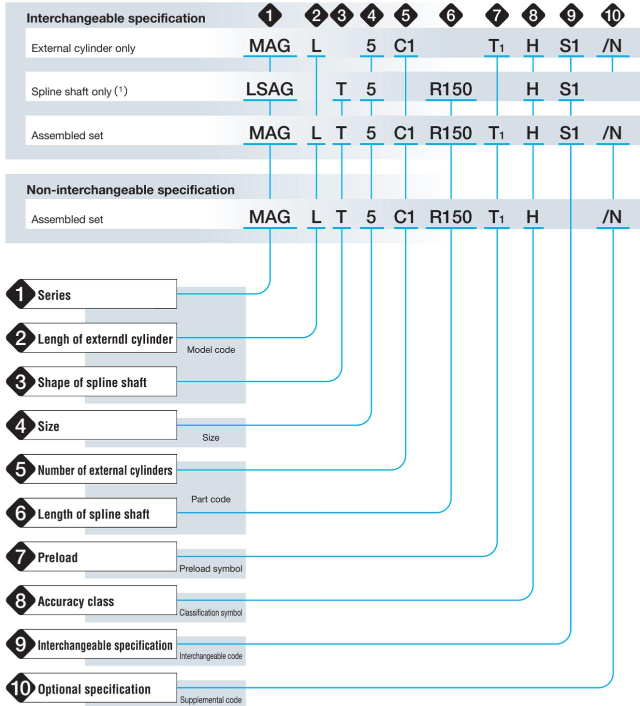
Note (1) : In case ordering spline shaft only, model code should be changed as LSAG (Solid shaft) or LSAGT (Hollow shaft).
