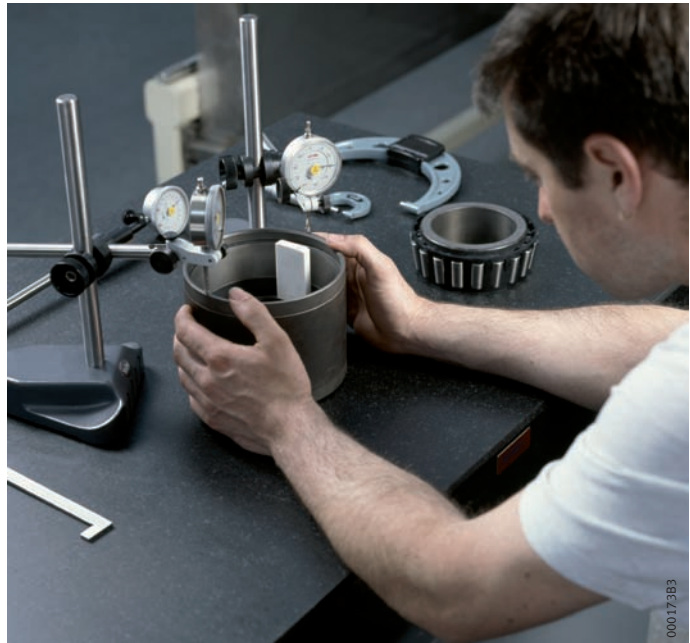
Figure 2 Measurement of TAROL components
