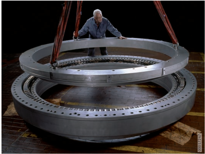
Figure 5 Mounting of new rolling bearing ring
