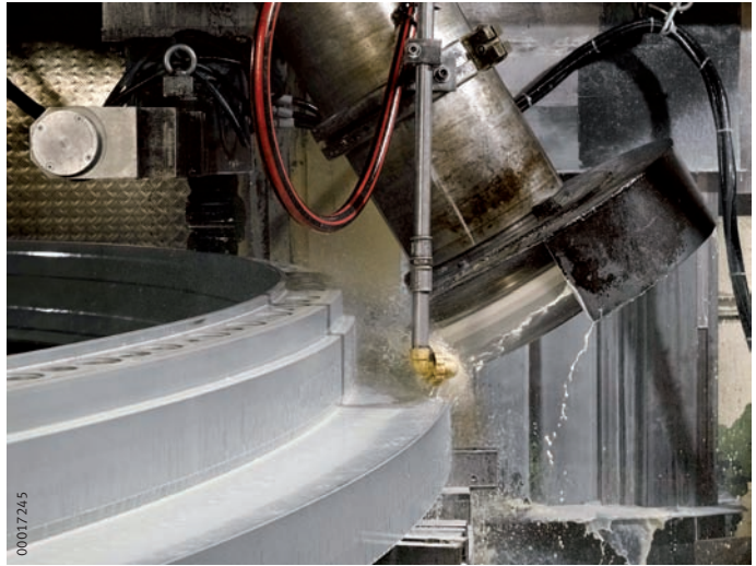
Figure 3 Regrinding of large size bearing ring
