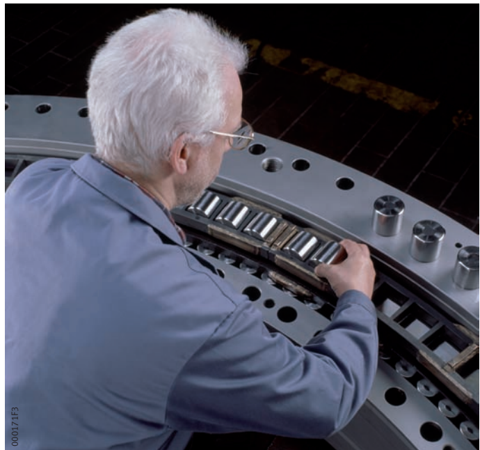
Figure 1 Assembly of a reconditioned rolling bearing for a tunnel boring machine
