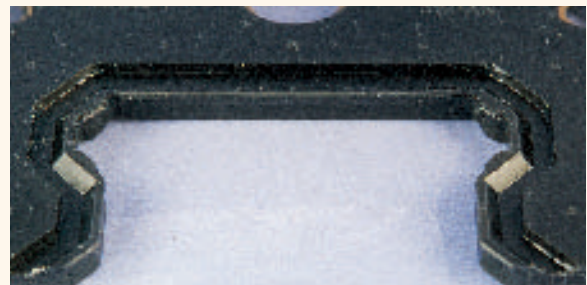
No.2 : LaCS installed on end seals: No abnormalities after traveling 5000 km
