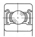
shields make no contact with the inner ring, they do not increase starting or running torque. Shields on stainless steel bearings are generally made from AISI 304 grade stainless steel.
