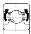
These seals are also made of *nitrile rubber* bonded to a metal washer but do not rub against the bearing inner ring and therefore do not have the same effect on bearing torque and maximum speed as contact seals so can be used for *low torque*, *high speed* applications. They offer superior protection over metal shields but do not provide as effective a seal as the contact type.
