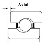
Clearance measured along the bearing axis is known as axial play. Axial play is approximately 10 times the radial play value.
