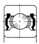
The standard bearing seal consists of *nitrile rubber* bonded to a metal washer. High temperature *teflon seals* (up to 250C) or *Viton seals* (up to 230C) are available on some sizes. The inner lip of the seal rubs against the bearing inner ring to provide an effective seal against smaller particles such as dust and moisture while preventing lubricant leakage. Contact seals produce much higher frictional torque levels than shields and reduce the maximum speed of a bearing.
