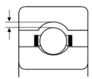
Also referred to as radial play, it is the amount of play or looseness between the inner and outer ring or more specifically: average outer ring raceway diameter minus average inner ring raceway diameter minus (2 x ball diameter). Radial play should not be confused with tolerance grade and is entirely separate.
