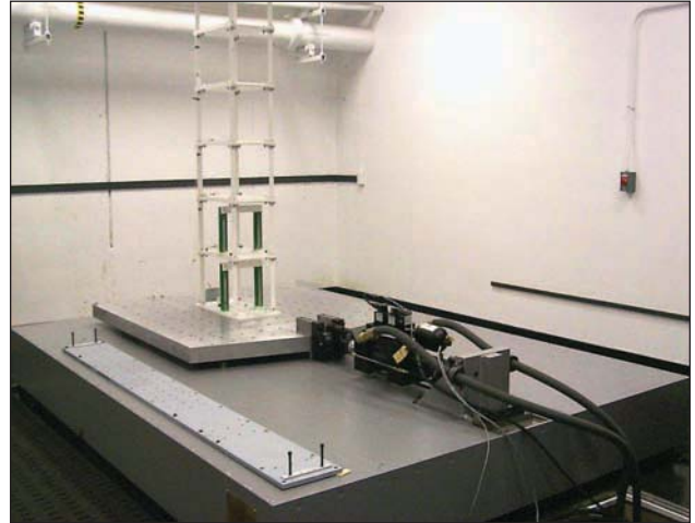
WUSCEEL shocktable used to measure effects of earthquakes on building structures.
